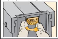
**5.** Retract the bolt just enough to remove the FIRE gauge. Reinstall the backplate. Retract the bolt just enough to insert the FIRE gauge and try to fire by pressing the butterfly trigger. The gun should not fire.
