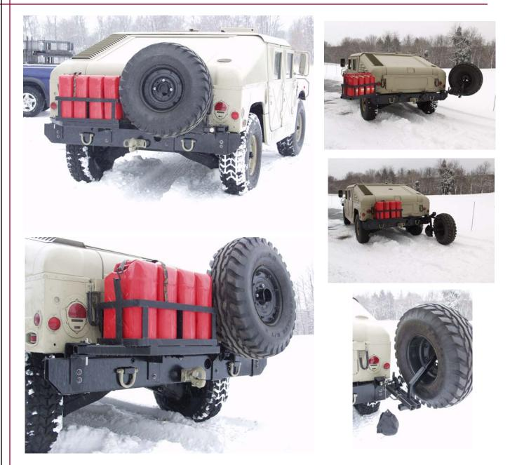
Ibis Tek can supply the accessories to allow you to modify a HMMWV equipped with or without an existing bumper to accept our Patented Mechanically Assisted Spare Tire Carrier (MASTC) and Jerry Can Holder (JCH). Both Systems rotate out of way of the back of the vehicle to access to the rear compartment :
